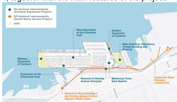
Figure 1 Overview and main features of Centerm Expansion Project (source: Port Authority web site)
